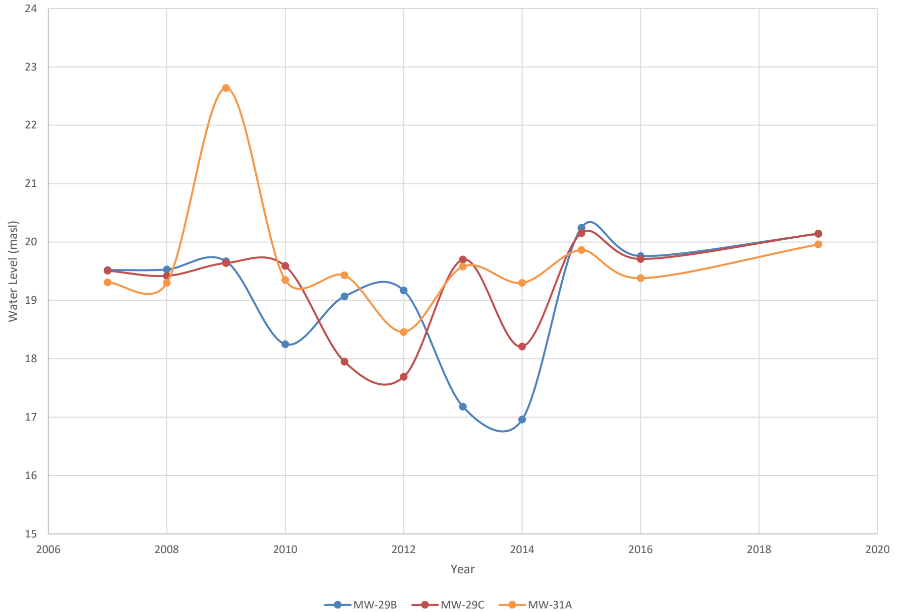
Figure D-11 - Historical Results of Groundwater Elevation in Upgradient Monitoring Wells
